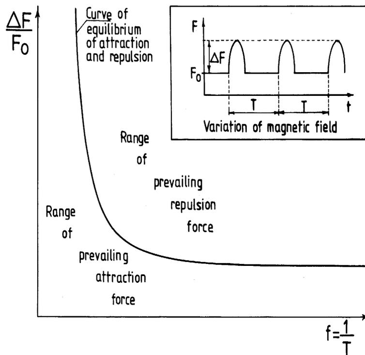
**Fig. #E2** ( $F_{12} z [1/5]$ ): The curve of the magnetic "interactions in equilibrium" between the magnetic field produced by a twin-chamber capsule (of Oscillatory Chambers) and all the ferromagnetic objects found in the range of this field. Originally this curve is shown in "Fig. F12" from monograph [1/5] and in "Fig. C12" from monograph [1/4].
