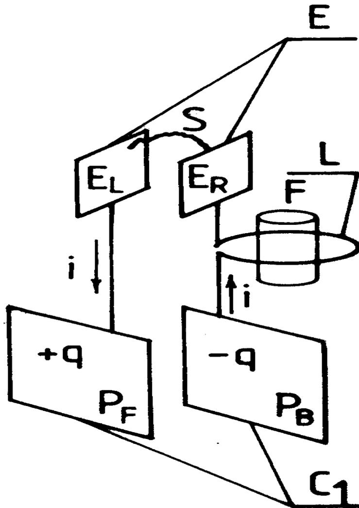
**Fig. #D1** (F1(a) in [1/5]): It shows a conventional form of an oscillatory circuit with a spark gap, as it was discovered by Joseph Henry in 1845. Its three vital elements (i.e. capacitance "C1", inductance "L" and spark gap "E") are provided by three separate devices, i.e.: by a capacitor "C1", by a coil "L", and by a pair of electrodes marked "E". Originally this drawing is shown as part (a) from Figure F1 in monograph [1/5].
